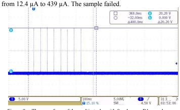
After 6-stroke the leakage current of sample B2 changes
