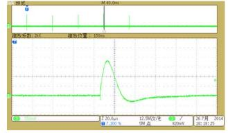
Figure 11. The waveform of the multi-stroke with 5 pulse with 50 ms interval
