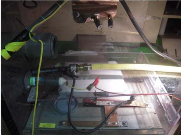
Figure 5. The 10/350 direct lightning experiment
