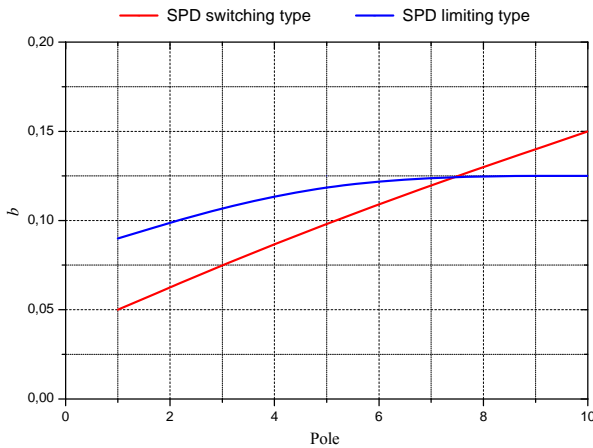
Figure 10. Values of coefficient b as a function of pole stricken for SPD1 switching and limiting type.
