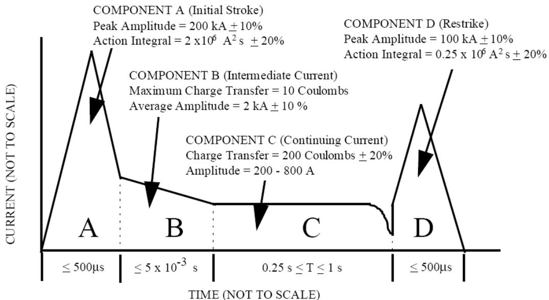
Figure 1. Representative lightning waveform. (After MIL-STD-464.)
