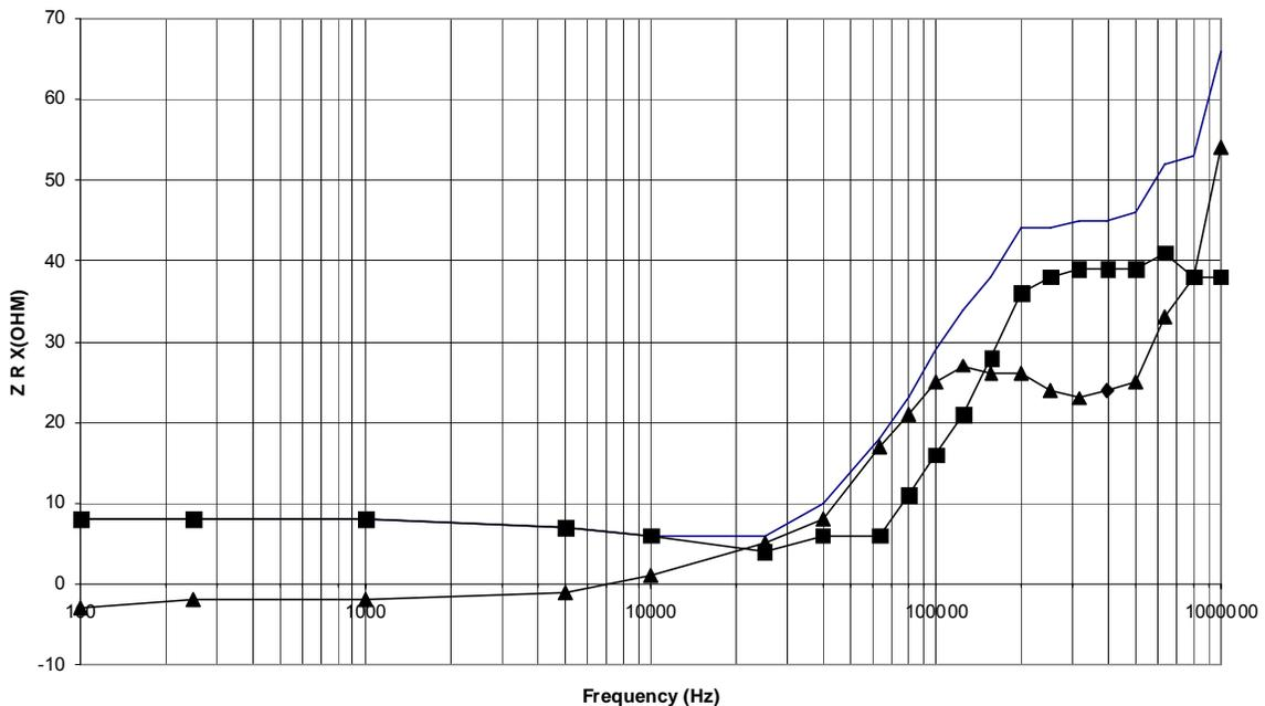
Figure 3. Impedance versus frequency plot for a ground mat consisting of 200 foot of 2/0 cable. Key: Impedance (◇), Resistance (■) and Reactance (△) as a function of frequency.
