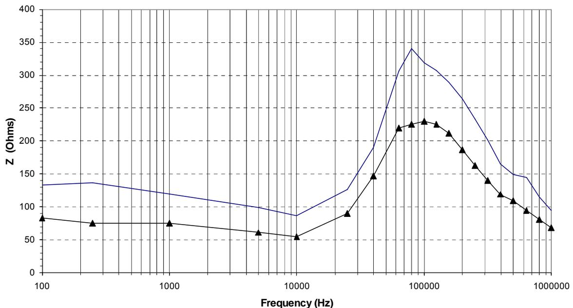
Figure 4. Impedance versus frequency for a 230 kV transmission line counterpoise with the overhead ground wire disconnected (straight line) and connected. (▲) (Data released courtesy of NEETRAC / Georgia Tech Management Board, Project No. 06-209.)
