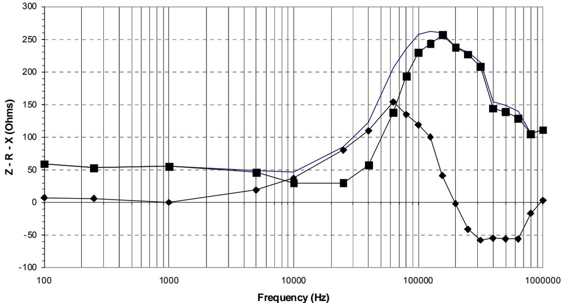
Figure 2. Single Ground Rod Impedance, Resistance and Reactance. Key: Impedance (-), Resistance (■) and Reactance (◇) as a function of frequency. (Data released courtesy of NEETRAC / Georgia Tech Management Board, Project No. 06-209).
