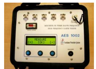
High Frequency earthing impedance meter
