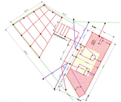
Earthing system model for an installation
