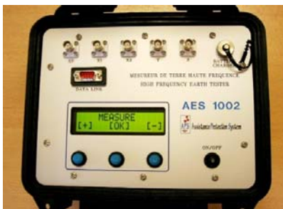
High frequency earth meter, Measurement results: Impedance variation related to frequency
