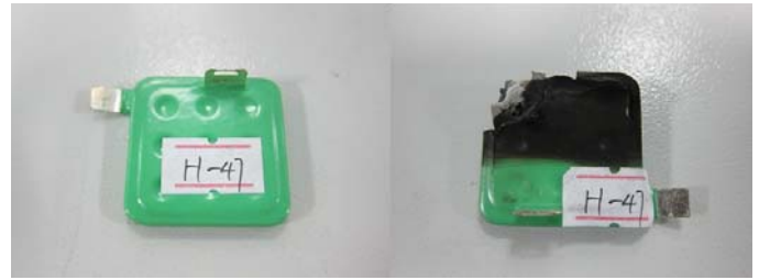
Figure 12 : sample H-47 is burned black after test
