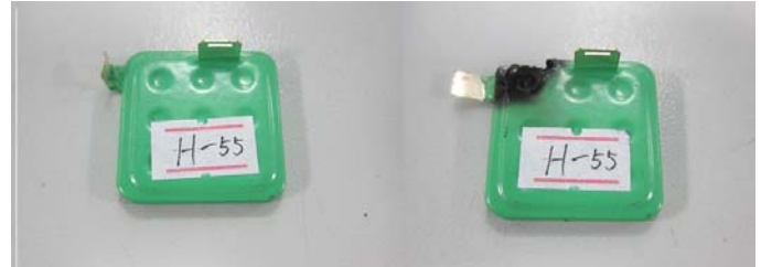
Figure 14 : sample H-55 burnt after test
