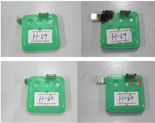
Figure 6 : example of tests results (puncture) with the surge tests
