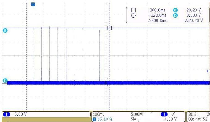
Figure 10. The waveform of the multi-stroke with 6 pulse with B2 sample
