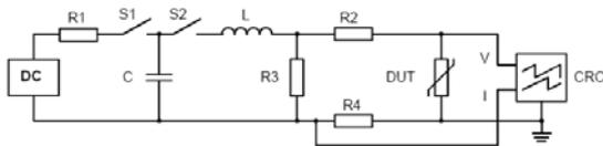
Figure 5. The diagram of the single-pulse current generator
