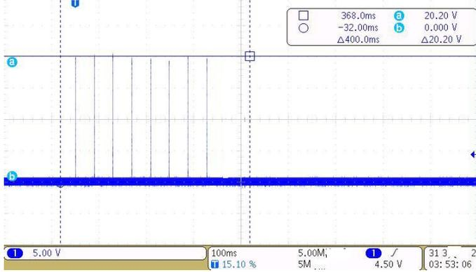
Figure 9. The waveform of the multi-stroke with 8 pulses on B1 sample
