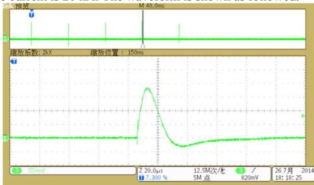
Figure 11. The waveform of the multi-stroke with 5 pulse with 50 ms interval
