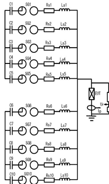
Figure 6. Diagram of the multiple pulses generator
