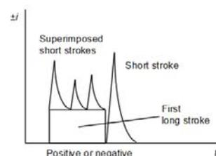
Figure 3. Possible multiple impulses for exposed areas or high structures
