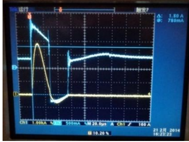
Figure 16. Oscillograms for two SPDs and lamp coordination test with 8 m - cable – Ispd3(yellow) and Ures3(blue)
