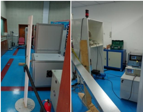
Figure 11. Coordination test for cables in metallic pipe and metal trays
