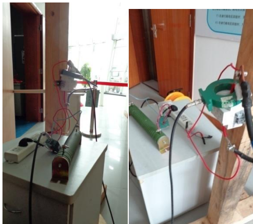
Figure 6. Test arrangement for resistive load
