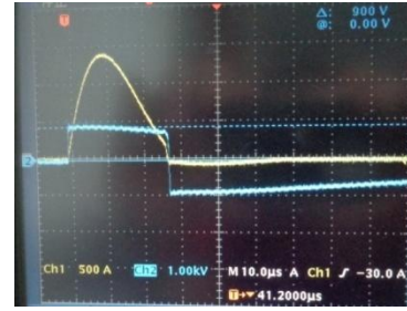
Figure 18. Oscillograms for two SPDs and lamp coordination test with 8 m - cable – Ispd3(yellow) and Ures3(blue)
